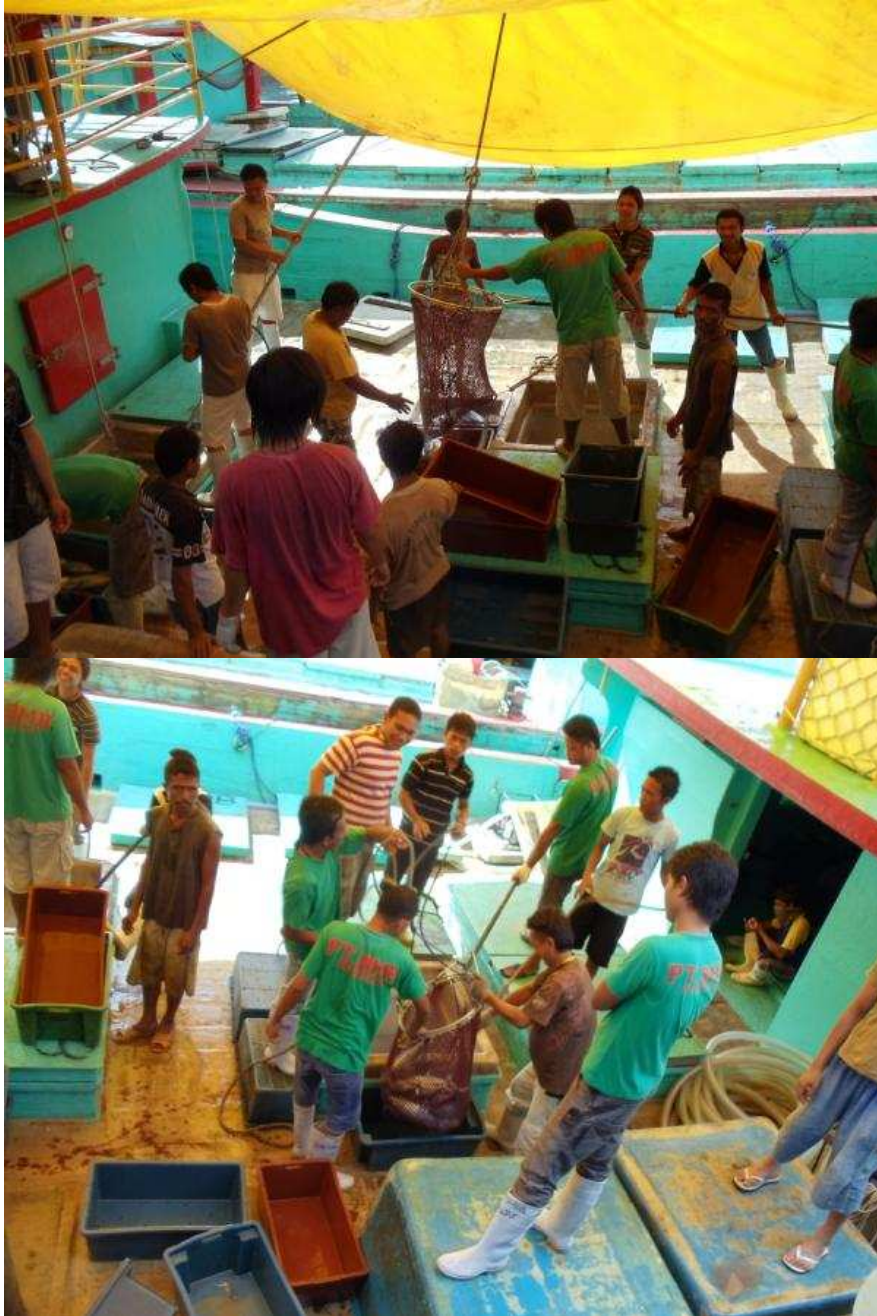
Photos 4 and 5. Unloading from the storage wells of a purse seine carrier at BMB wharf in Bitung. The small brail is lowered into the holds and the (unsorted) catch is scooped up and poured into plastic baskets on the deck. Catch unloaded from the carrier vessels was typically around 150t.
